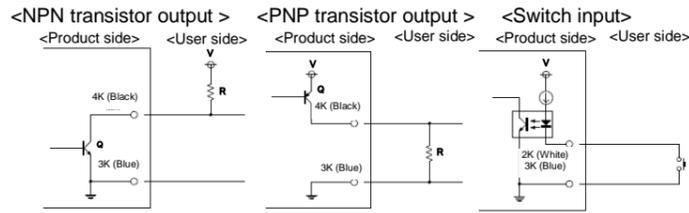
\*Press F2 to set to Switch input (Remote zero adjustment and Accumulated output reset).
