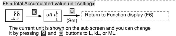
The current unit is shown on the sub screen and you can change it by pressing  $\Delta$  and  $\nabla$  buttons to L, KL, or ML.
