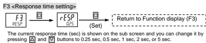
The current response time (sec) is shown on the sub screen and you can change it by pressing  $\Delta$  and  $\nabla$  buttons to 0.25 sec, 0.5 sec, 1 sec, 2 sec, or 5 sec.
