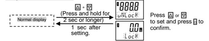
\* While key lock is enabled, any other operations than key lock operation are disabled. Disable the key lock in the same method. When you press a key while key lock is enabled, "LOCK" is shown on the sub screen for 2 seconds.
